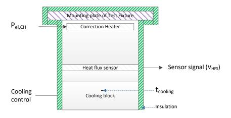
Figure A-2: Calibration of the heat flux measurement setup.
