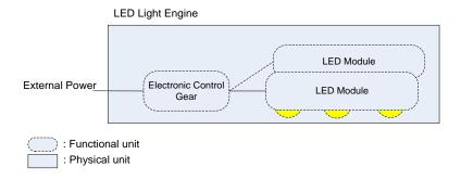
Figure 2-3: Schematic overview of a LED Light Engine with Integrated ECG
