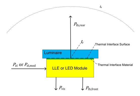
Figure 6-1: Thermal model of a LLE - Luminaire or a LED Module - Luminaire combination
